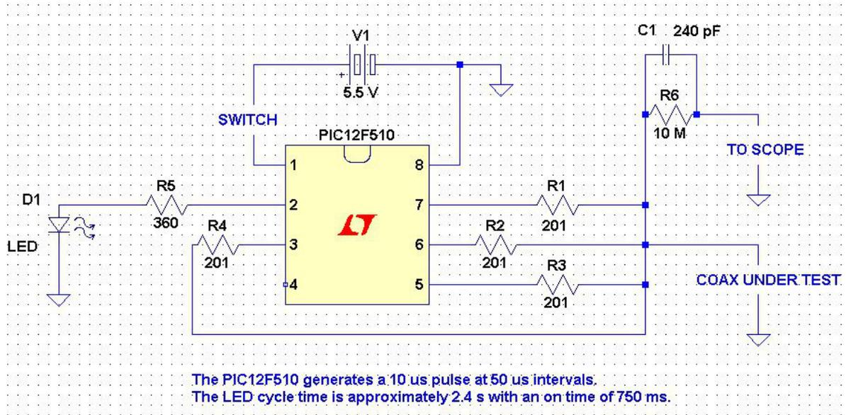
**Figure 5. Schematic of TDR pulse generator.**
