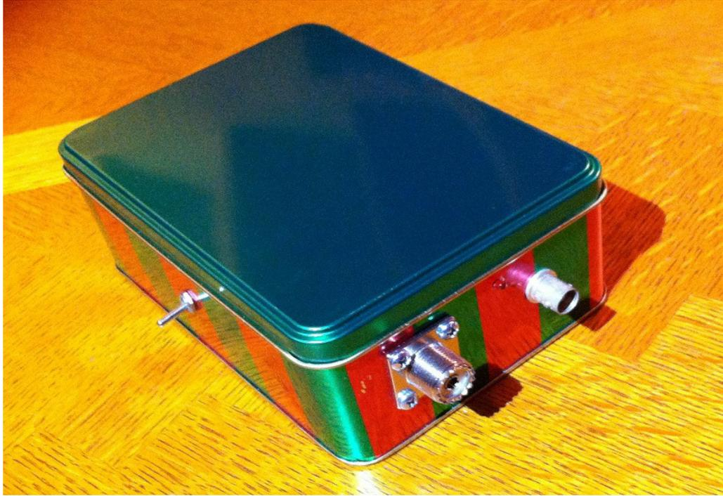
**Figure 3. Completed TDR pulse generator housed in a Christmas tin.**
