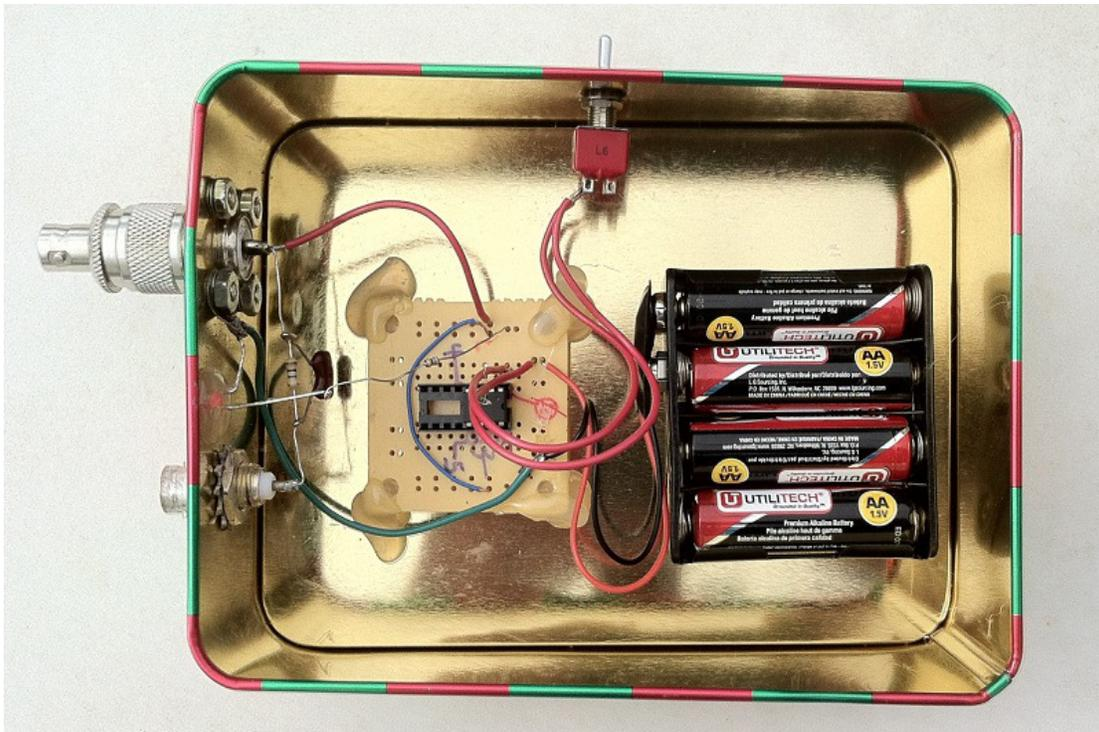
**Figure 4. Inside completed TDR pulse generator..**
